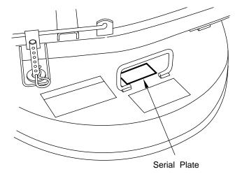
Figure 1-1 Mower Deck Serial Plate Location
